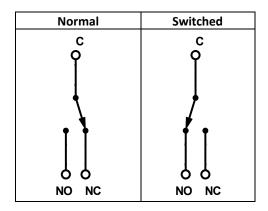
3.1.2 The 0729-1763-XX uses relays with 2 connections, COM and NC/NO. The function will depend on the polarity. When polarity is 0, the NC/NO connection functions as the NC connection. When polarity is 1, the NC/NO connection functions as the NO connection. This function is shown below:
