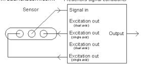
Caution!-Ensure that all test and operating circuits are entirely free of direct current. Direct current will cause level damage and/or instability.
