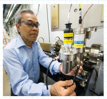
than typical cold cathodes (down to 1\*10<sup>-11</sup> Torr), allowing accurate UHV measurement critical to APS-U. The easy cleanability means that the gauge will last indefinitely in an application like that of APS-U, where equipment must remain in operation for decades at a time with little or no intervention from operators.
