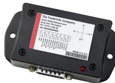
The RS232 interface link is thru the black wire (input, 14) and the brown wire (output, 6). Pins 1, 9, and 15 are ground. The connector on the unit is a male DB15 connector.
