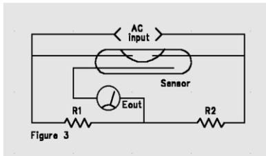
**Caution!-Ensure that all test and operating circuits are entirely free of direct current. Direct current will cause level damage and/or instability.**
